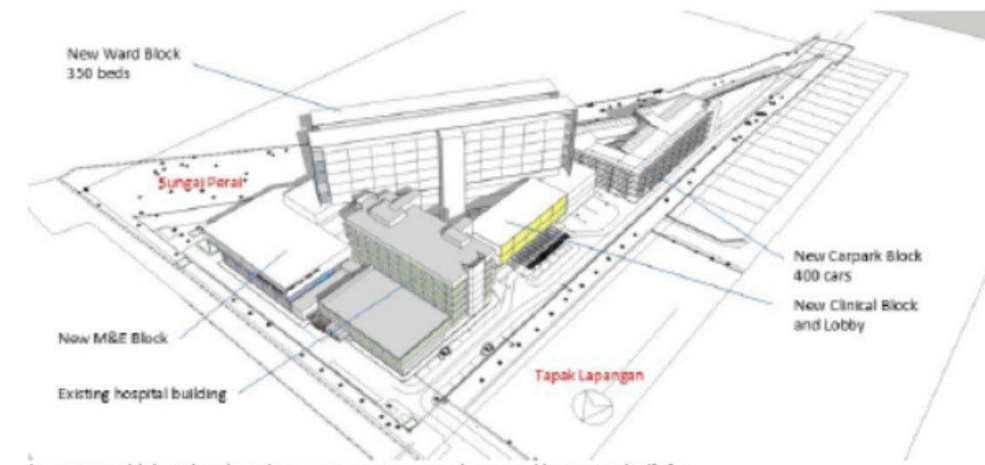
Isometric view of the hospital complex, used to manage construction sequence, demarcation of departments and traffic flow.
