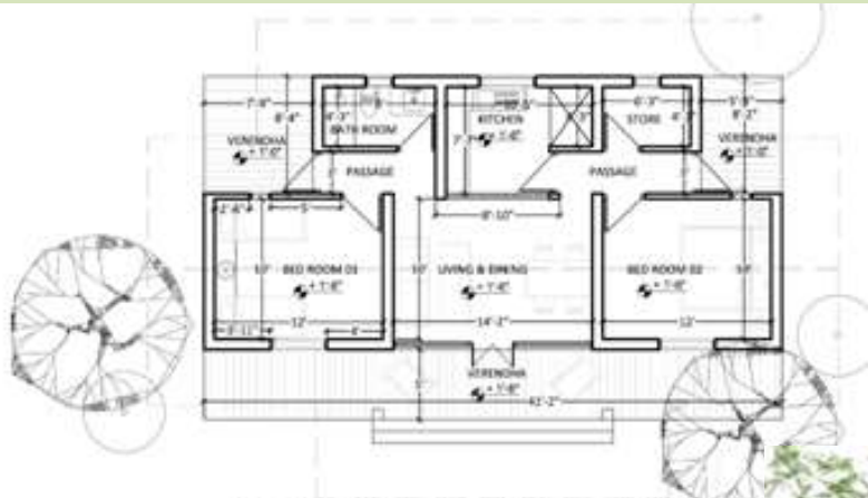
GROUND FLOOR PLAN SCALE : 8 FT TO AN INCH AREA : 908.60 Sq.ft AREA : without verandah : 600.00 Sq.ft
