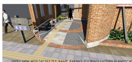
ENTRY VIEW WITH TACTILE TILE, RAMP, RAILING, FLOORING PATTERN & LANDSCAPE
