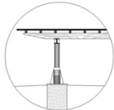
Bamboo and steel Joint detail
